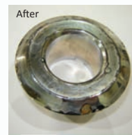
Chrome and plastic parts after 100 hours of testing.
